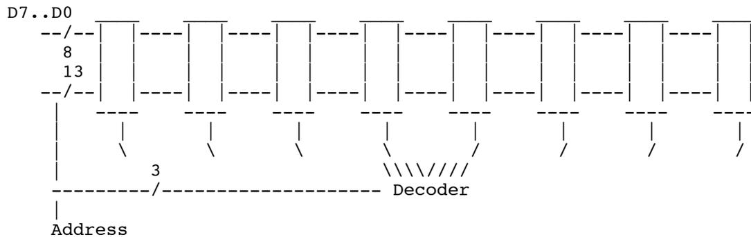
The correct chip is selected by the decoder on the basis of the high 3 bits of the address. The outputs of the decoder go to a "chip select" input on each chip.
